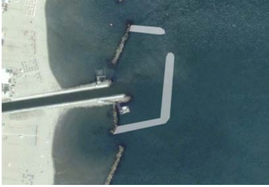
Figure 5. Access channel to Casal Borsetti Marina. The harbour extension is given with a gray line.
