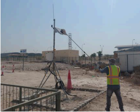
Figure 2. Actual underground temperature monitoring setup at the outdoor test facility
