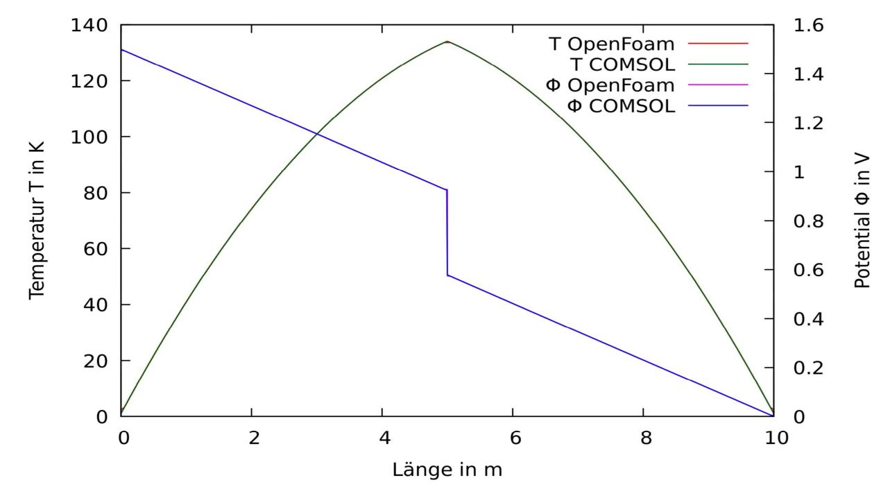
The main objective of the project was to examine and compare the capabilities and performance of OpenFOAM and COMSOL Multiphysics in accurately and efficiently analyzing contact resistance.
