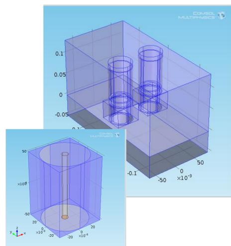
**Figure 2.** The full model based on the microcalorimeter (back) and the simplified section used for this study.
