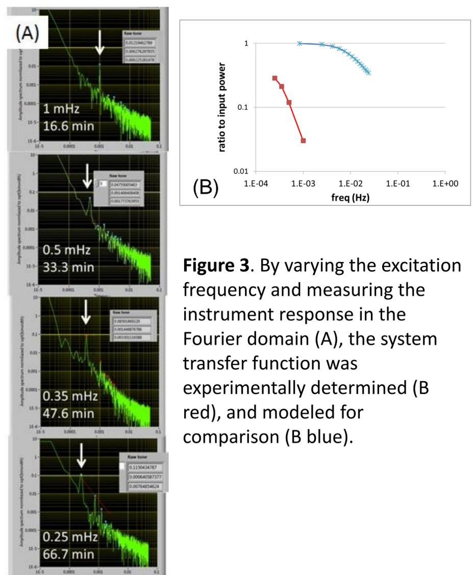
**Figure 3.** By varying the excitation frequency and measuring the instrument response in the Fourier domain (A), the system transfer function was experimentally determined (B red), and modeled for comparison (B blue).
