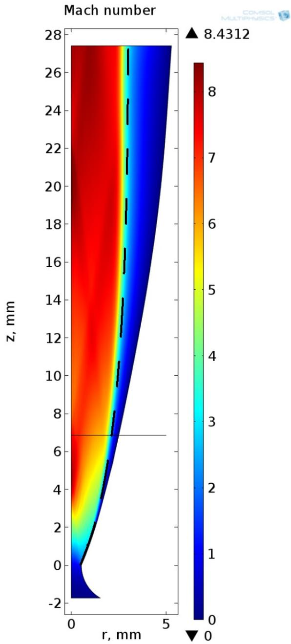
**Figure 1:** Mach number distribution in the nozzle. The dashed line indicates inviscid solution
