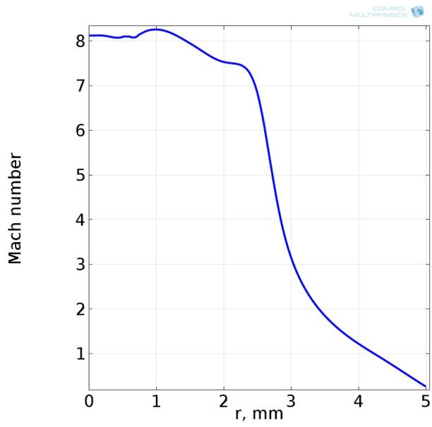
**Figure 2:** The radial Mach number distribution in the exit plane
