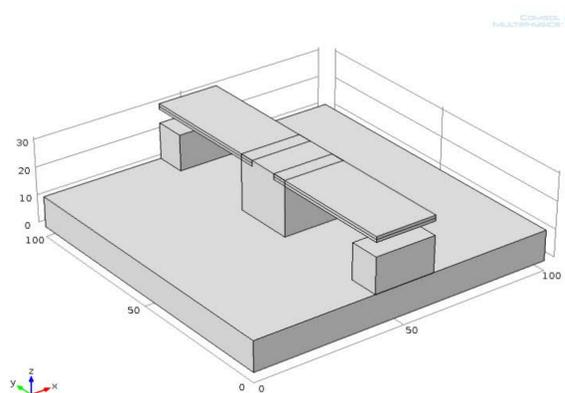
**Figure 1: Model of bolometer**
