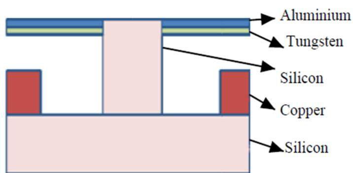
**Figure :2 structural details of bolometer**
