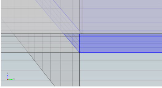
Figure 3: Mesh distribution in the PCM.
