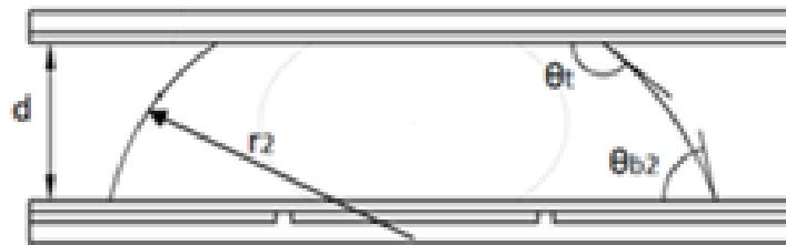
(b). (B-B') section view (c). (A-A') cross-section view Figure 4. Mechanism of droplet splitting [10]
