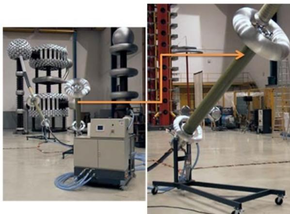
**Figure 1:** The Cable Termination (CaTr)- Right and CaTr System being used in high-voltage AC test system- Left.
