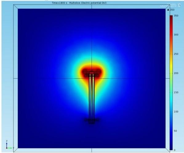
**Figure 2:** Electric Potential plot for the applied 350 kV D.C.
