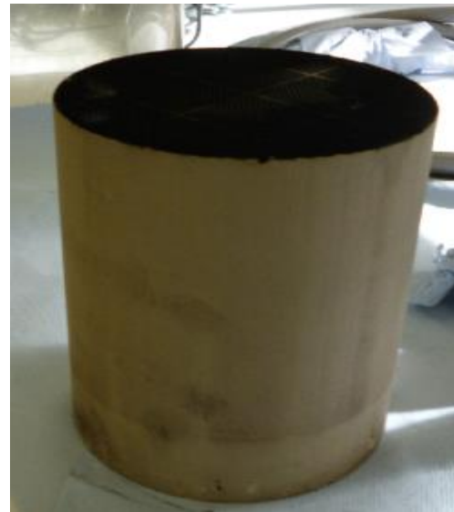
The soot loaded DPF before regeneration Mass- 1849g
