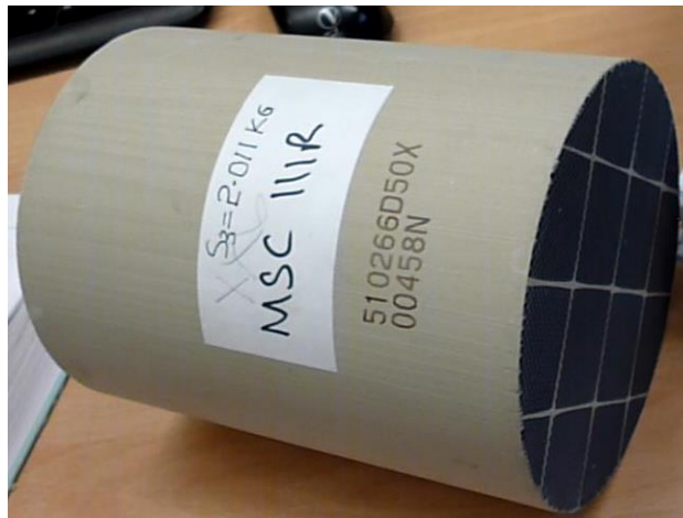
JM SiC non-catalyzed DPF Length = 18.2cm, Diameter = 14.4cm Mass – 1830 g
