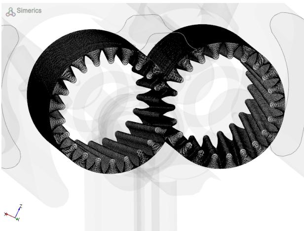
Figure 1: External helical gear pump CFD analysis.
