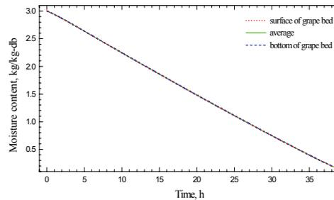
**Figure 3.** Evolution of grape moisture content during the drying process.
