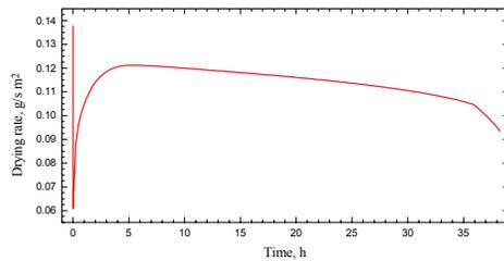
**Figure 4.** Drying rate vs. drying time for grape dehydration.
