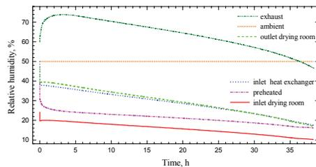
**Figure 6.** Relative humidity of drying air at different locations vs. drying time.
