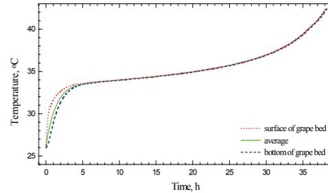
**Figure 2.** Evolution of grape temperature during the drying process.
