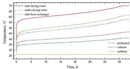
**Figure 5.** Drying air temperature at different locations vs. drying time.
