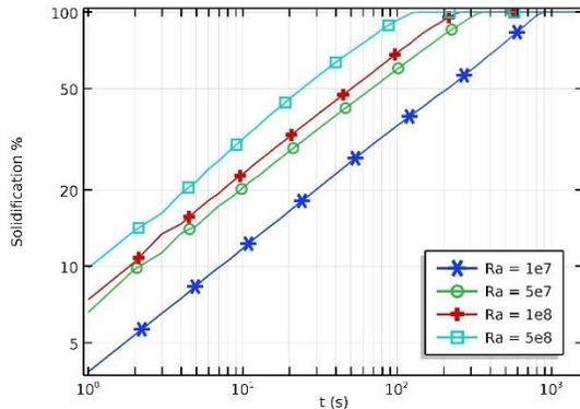
**Figure 3.** Solidification percentage vs. time, at different values of Rayleigh number for the 25% filling case.
