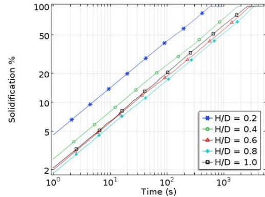
**Figure 5.** Solidification percentage vs. time for different filling percentages at  $Ra = 10^7$ .
