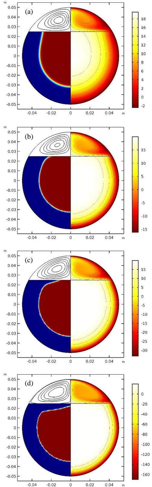
**Figure 2.** Phase (left) and temperature (right) contours for  $Ra = 10^7, 5 \times 10^7, 10^8,$  and  $5 \times 10^8$ , for the 75% filling case.
