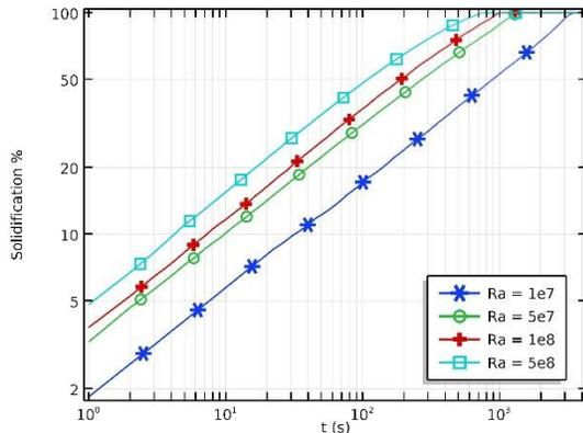
**Figure 4.** Solidification percentage vs. time, at different values of Rayleigh number for the 75% filling case.
