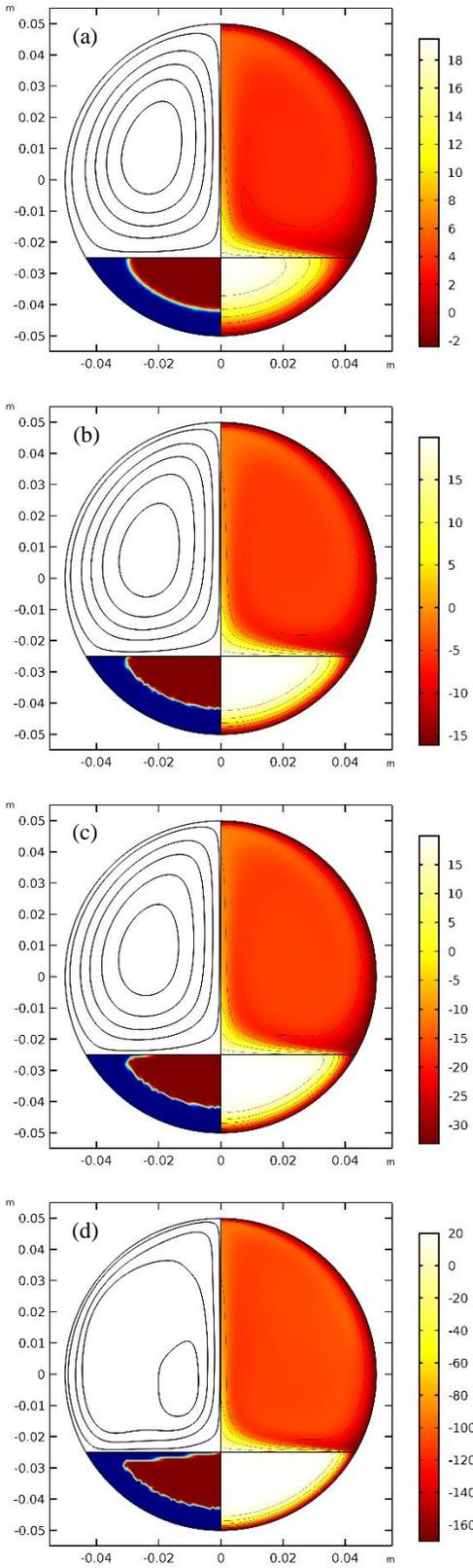
**Figure 1.** Phase (left) and temperature (right) contours for  $Ra = 10^7, 5 \times 10^7, 10^8,$  and  $5 \times 10^8$ , for the 25% filling case.
