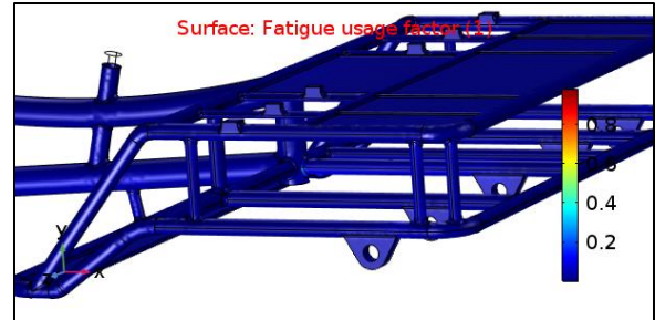
Figure 9. Passenger/load area, Stress-Based Findley model, horizontal load case.
