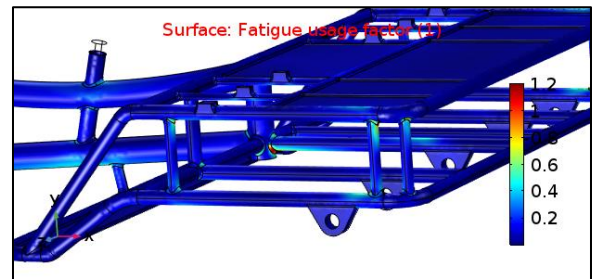
Figure 10. Passenger/load area, Stress-Based Findley model, vertical load case.
