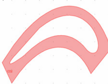
Figure 2. 2D Representation of the main section of the galvanic cell realized for deposition on turbine vane.
