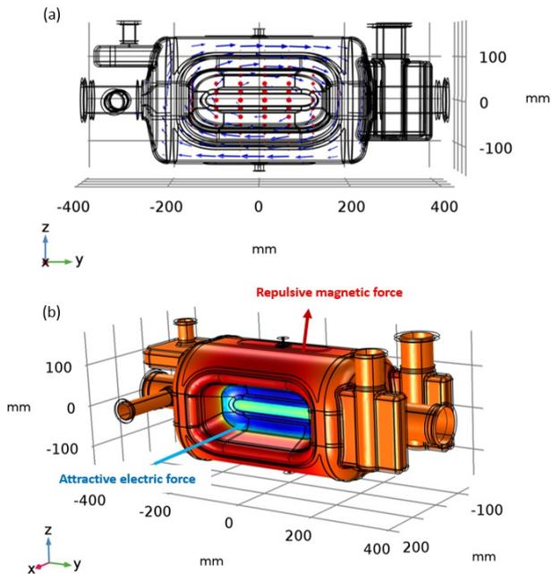
**Figure 1:** (a) Magnetic (blue) and electric (red, pointing in the negative x direction, towards the paper) field vectors for the fundamental mode of the RFD superconducting cavity. (b) Electromagnetic pressure on the cavity interior walls for the RF fundamental frequency, used for Lorentz force detuning calculations.
