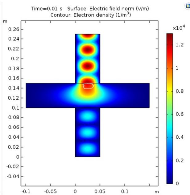
**Figure 1:** Electric Field is an important factor regarding ignition of the plasma flame and sustainability. When critical electron density is reached, waves no longer penetrate that area.
