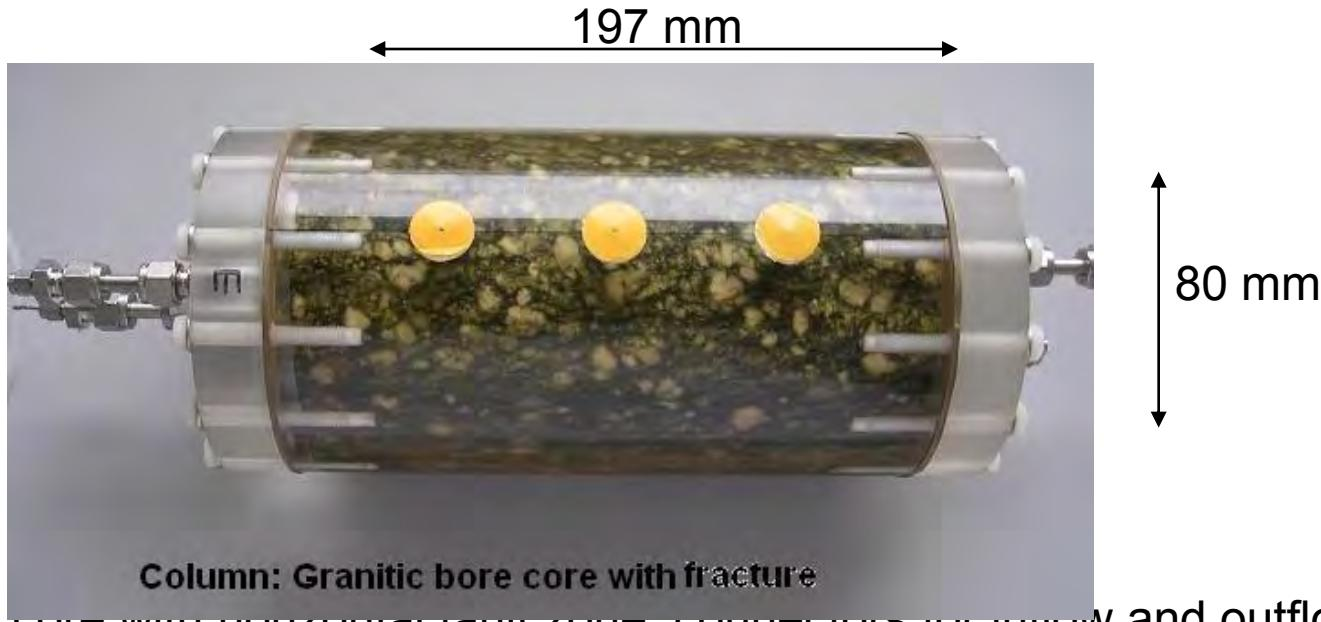
Granitic drill core with horizontal fault zone, connectors for inflow and outflow, plexiglass casing, flow through experiment (0.1ml/min)
