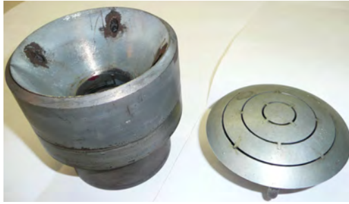
Figure 2. The phase plug is made of several parts making up the throat and the slits.
