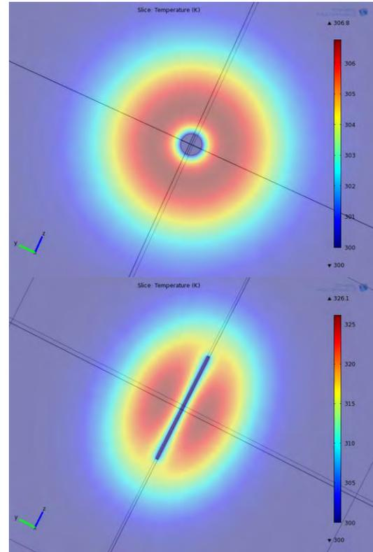
**Figure 1.** Cross-Sectional view of thermal response for a gold nanosphere (top) and gold nanorod(bottom).
