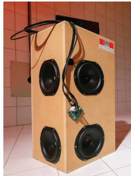
FIGURE 1. Active Electroacoustic Resonator prototype. Image credit: EPFL/Alain Herzog.
